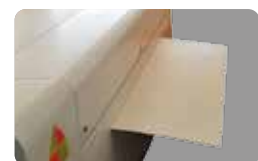
Fig. 4 - Machine rear open for materials larger than the work area
